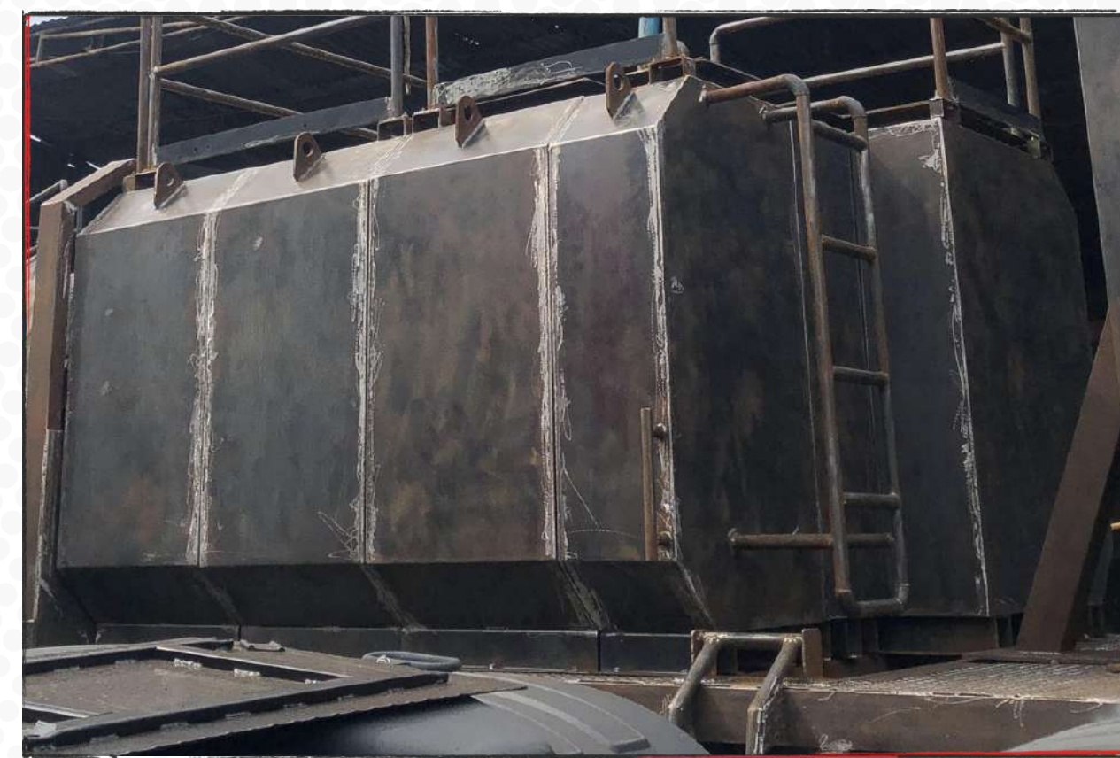
Lube Oil Tanks PT. Sasmaka Lestari Karya
